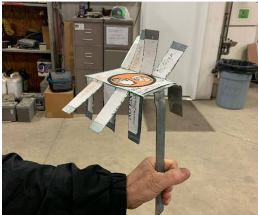
Figure 1. Water sensitive tape was attached to each tab on the contraction to simulate spray coverage on either sugarbeet or waterhemp.
